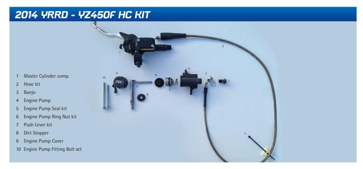
New kit for the 2014 YZ450F model, as used in GP by factory riders and others. Improves functioning of the clutch and especially the clutch plates' durability. Automatically adjusts the clutch free play, avoiding the rider having to do it manually.
